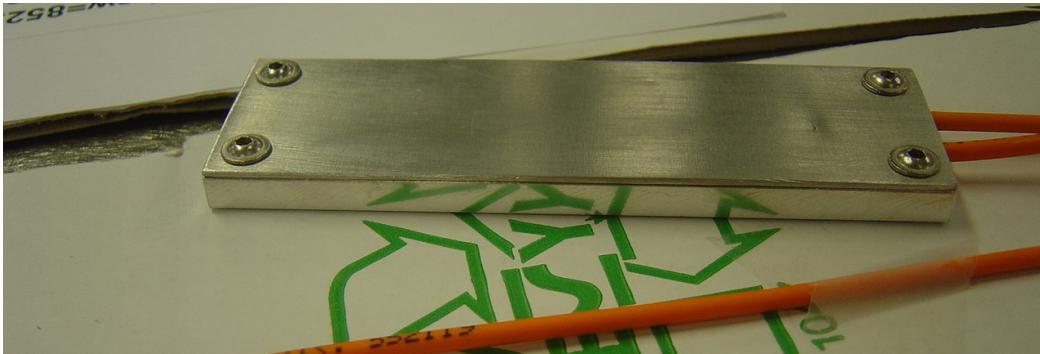
Figure 2: temperature sensor with aluminium encasing
